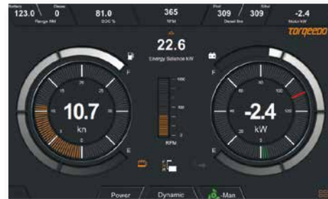
Drive screen: All important information needed while motoring. You can choose to display or hide the information line at the top.
